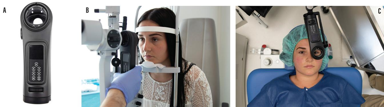
Figure. The C-Eye device (A) fits on a large variety of Haag-Streit and Carl Zeiss Meditec slit lamps (B). It can also be used with a table mount accessory in the OR (C).
